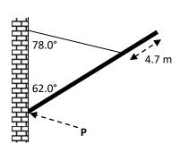
4. A heavy uniform plank of mass 55 kg and length 4.8 m is attached to a wall hinge and pulled upward by a force of  $4.6 \times 10^2$  N as shown below. What is the net torque on the plank in the horizontal position shown?
